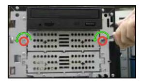
2. From the side of the drive bay, slide the drive bay lock by pushing it to the left to release the drive lock bar.
